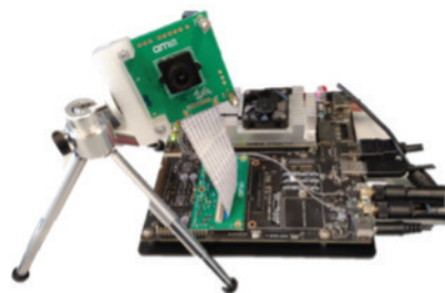
AMS demo kit. The NIR-enhanced sensor combined with a NIR light source shows the capability to detect drowsiness of a car driver, sending a warning signal.
