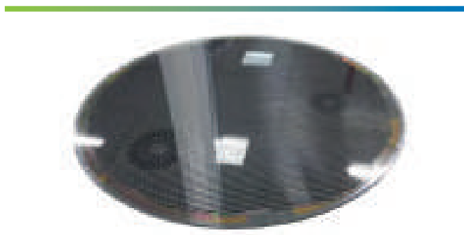
Wafer-level hermetic sealing of more than 5000 infrared sensor chips under deep vacuum Copyright XFAB
