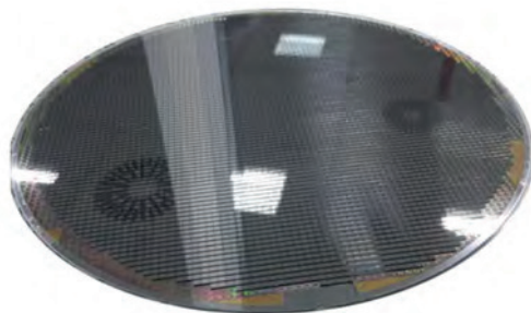
Wafer-level hermetic sealing of more than 5000 infrared sensor chips under deep vacuum Copyright XFAB
