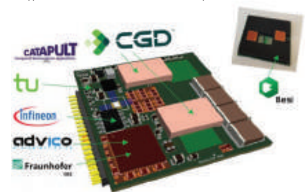
Figure 1: GaNext GaN IPM Development. CGD developed the GaN chip, Infineon developed Gate Driver, Advico and Fraunhofer IMS developed the Si Controller, TU Dortmund conducted the design of PCB power electronics, Besi developed the encapsulation for the IPM and CSAC conducted application testing.
