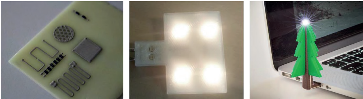
Examples of hybrid manufactured electronic structures: in-plane, embedded and 3D structures Photo credit: Bosch, Philips Lighting and Neotech
