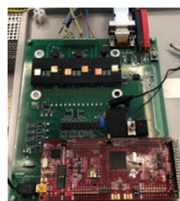
Figure 10: MACCON's GaNext Demonstrator for Motor Drives Applications (left) that extends voltage range of 40kHz inverter portfolio by factor of 5 (right). ©MACCON
