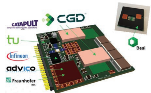
Figure 1: GaNext GaN IPM Development. CGD developed the GaN chip, Infineon developed Gate Driver, Advico and Fraunhofer IMS developed the Si Controller, TU Dortmund conducted the design of PCB power electronics, Besi developed the encapsulation for the IPM and CSAC conducted application testing.
