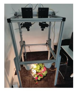
ImVia & MsEyeTech solution. Two single-shot MS cameras cover the VIS and NIR spectrum.
