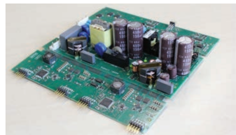
Figure 9: The technology to reduce the size of the output stage by increasing the switching frequency has been transferred from Signify research to Signify product development to be implemented in commercial products within one year from now. ©Signify
