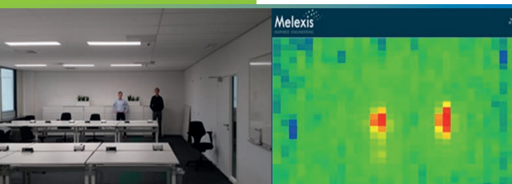
Demonstrator of an IR People Detection Sensor for smart building applications
