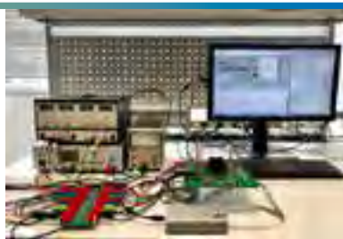
IEEE 1687 demonstrator based on a SOC processor silicon product
