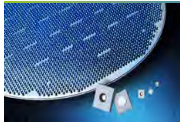
Demonstrator of a cap wafer with more than 5000 silicon lenses on a wafer
