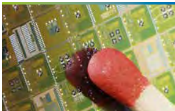
Illustration of the integrated AlScN pyroelectric elements on a CMOS-MEMS wafer
