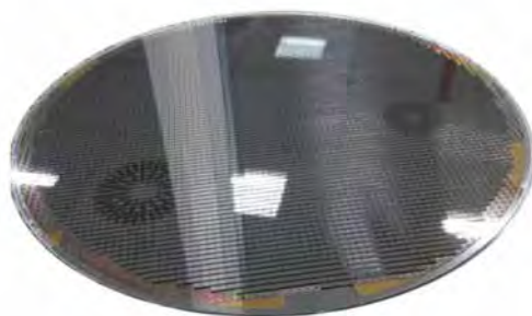
Wafer-level hermetic sealing of more than 5000 infrared sensor chips under deep vacuum Copyright XFAB
