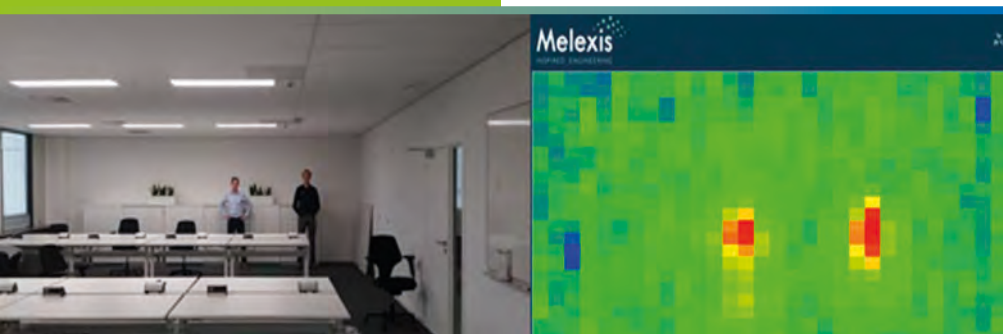
Demonstrator of an IR People Detection Sensor for smart building applications
