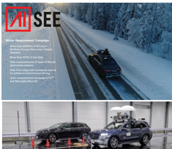
● Figure 3. Winter testing campaigns on public roads (top) and validation campaigns in controlled environment (bottom). Copyright Mercedes-Benz
