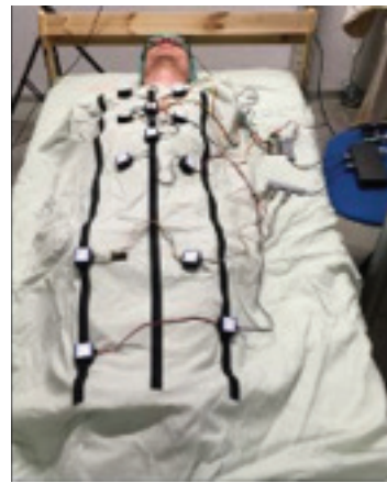
Figure 3: Motion sensing blanket (source: TU/e)
