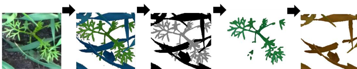
Fig. 1. Separation of crop and weed using the proposed algorithm (More details: https://www.youtube.com/watch?v=dNR4dE2Cp_M&t=2s ).
