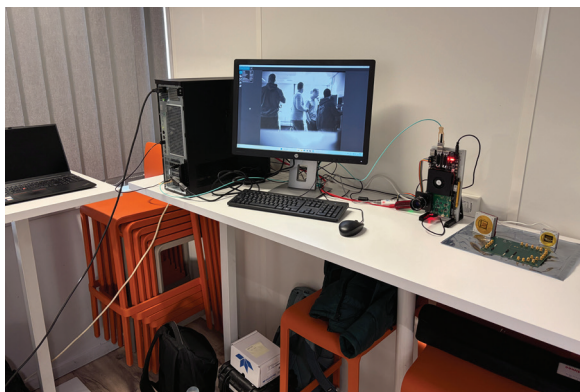
Figure 6: Demo 10 Gpix/s camera and 100 Gb/s transmission via CoaXPress. IMAGINATION consortium (taken at the final review meeting)
