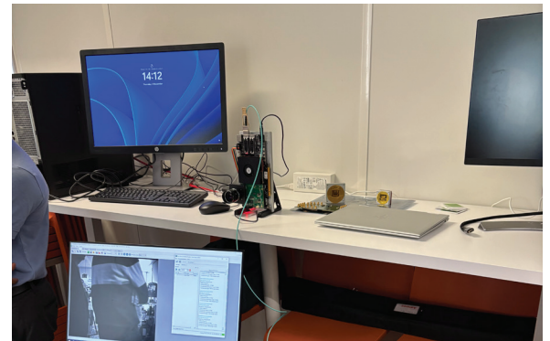
Figure 7: Demo 10.5 GB/s vision board with new Euresys frame grabber and Teledyne Adimec camera. IMAGINATION consortium (taken at the final review meeting)
