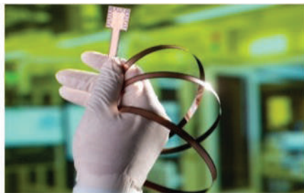
● Figure 3. HyPerStripe manufactured with R2R process, at Fraunhofer EMFT, EMFT
